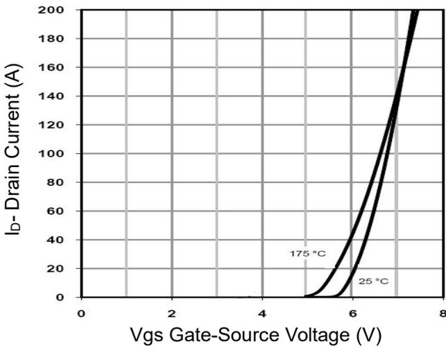
**Figure 2 Transfer Characteristics**
