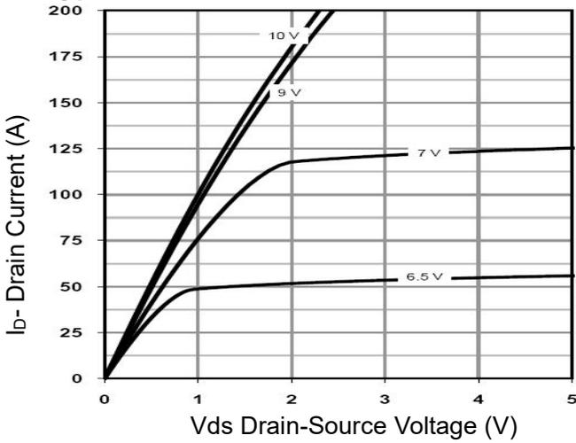
**Figure 1 Output Characteristics**
